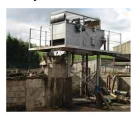
The Groundhog slurry separator from **Pollution Control** and the similar unit from **NC Engineering** are in the former camp, and have two fixed concave screens with sweeping elements working on the inner surface.
