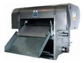
The Carier Rotoscreen separator from Linton Solutions also squeezes liquid from solids. But in this case there are two pairs of rollers, one on the inside and one on the outside of a rotating barrel screen.
